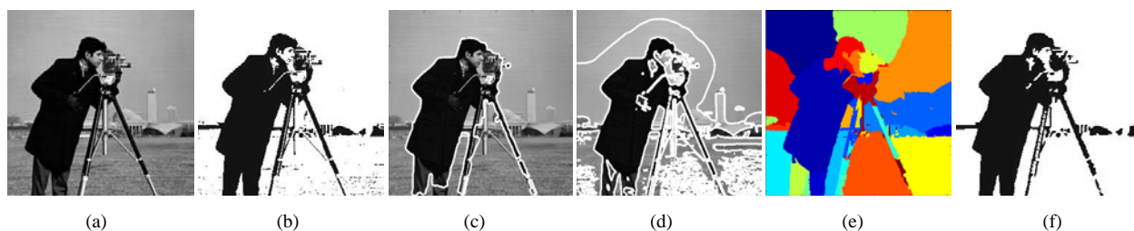
Fig.6. Original cameraman image and the segmentation results. (a) Original image; (b) segmentation by Otsu thresholding; (c) segmentation by LSEWRI; (d) segmentation by RACM; (e) segmentation by MNCut; (f) segmentation by HDSS-1.
