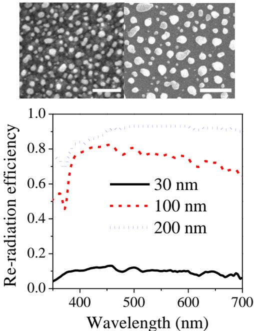
**Figure 3.** SEM images of the annealed silver films on ITO (top left) and on silicon (top right) surfaces. Scale bars denote 1 micron. DDA simulation results of the re-radiation efficiency dependence on the particle size (bottom).
