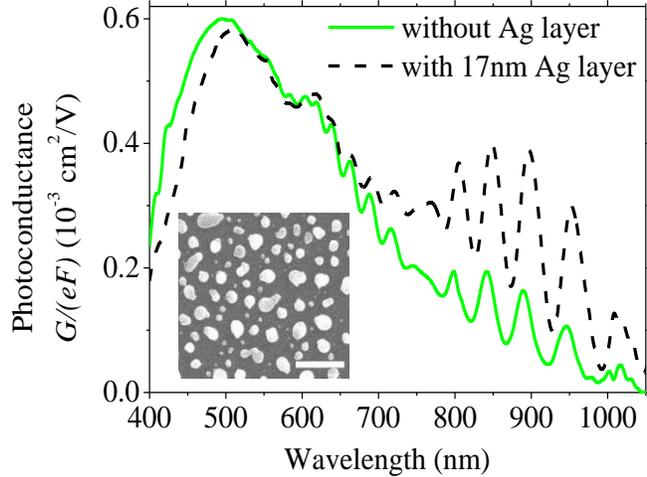
**Figure 2.** Normalized photoconductance spectra of the SOI photodetector with and without annealed silver film. Inset shows the SEM image of annealed silver films on the silicon layer with 1 micron scale bar.
