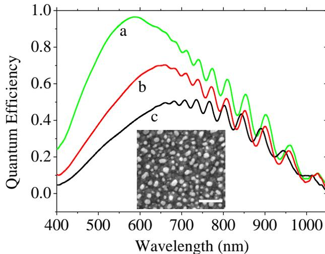
**Figure 1.** QEs of a nc-Si:H solar cell before and after deposition of annealed silver films; (a) as received (b) annealed without silver layer (c) with annealed silver film. Inset shows the scanning electron microscope (SEM) image of annealed silver films on top of ITO layer with 1 micron scale bar.
