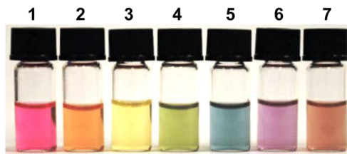
FIG. 1. (Color online) Multicomponent plasmonic nanogels with tunable optical properties. (1) 13.3 ppm Au(S, d=30 ), (2) 8 ppm Au(S, d=30 ) + 10 ppm Ag(S, d=35 ), (3) 13.3 ppm Ag(S, d=35 ), (4) 10 ppm Ag(S, d=35 ) + 10 ppm Au (R, \alpha=2.3 ), (5) 13.3 ppm Au (R, \alpha=2.3 ), (6) 10 ppm Au(S, d=30 ) + 10 ppm Au(R, \alpha=2.3 ), and (7) 6.7 ppm Au(S, d=30 ) + 6.7 ppm Ag(S, d=35 ) + 5 ppm Au (R, \alpha=2.3 ). S and R denote spherical and rod-like NPs, respectively.
