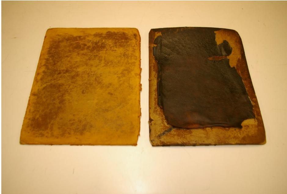
Leather covered boards from the same book depicting water damage and subsequent blackening to the board on the right; the leather became extremely brittle on drying and also suffered some degree of shrinkage. This type of damage is irreversible and will necessitate rebinding.
