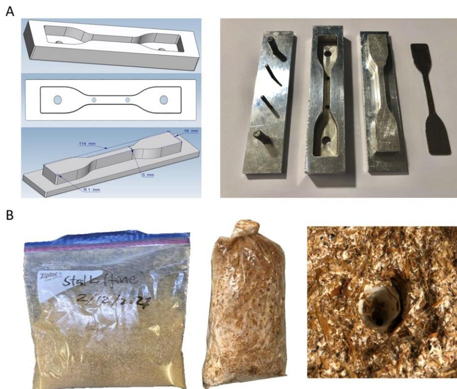
**Figure 5-2. A.** Mold design drawing (left) and model(right) **B.** Three different materials: stalk (S), stalk with mycelium (SM), and hardwood mixed with coffee grounds with mycelium (HCM) (from left to right.)
