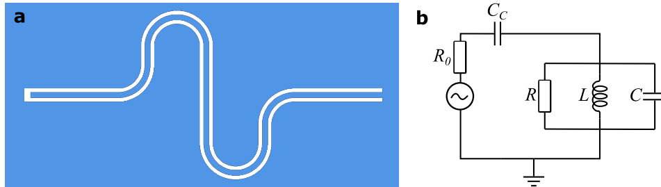
Figure 9: (a) Quarter-wave resonator comprised of a CPW transmission line with one end open and one end shorted to ground. (b) Near resonance, the quarter-wave CPW can be modeled by a simple driven parallel RLC circuit.
