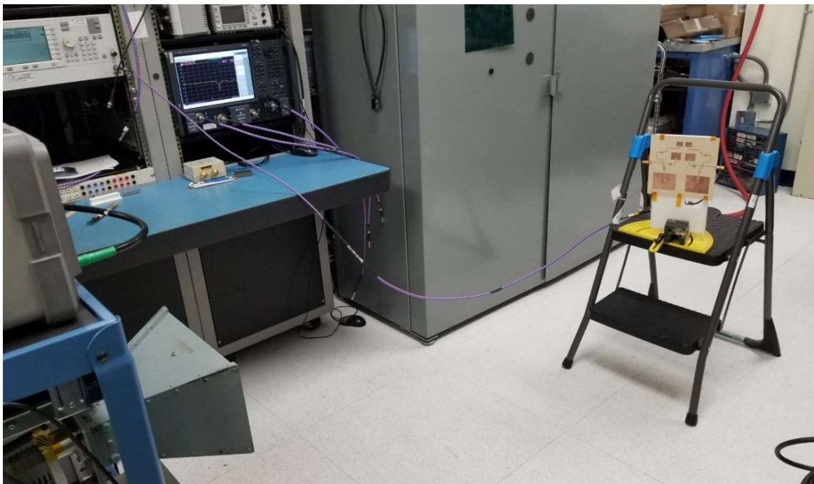
Figure 4-19 1D multiplexed antenna array radiation pattern test setup.
