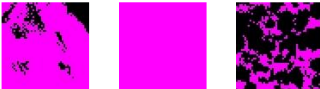
Figure S4. Raman maps of 0.6M NaCl indicating the presence of hydrohalite. Maps were taken at -27.9^{\circ}\text{C} , -31.9^{\circ}\text{C} , and -29.6^{\circ}\text{C}
