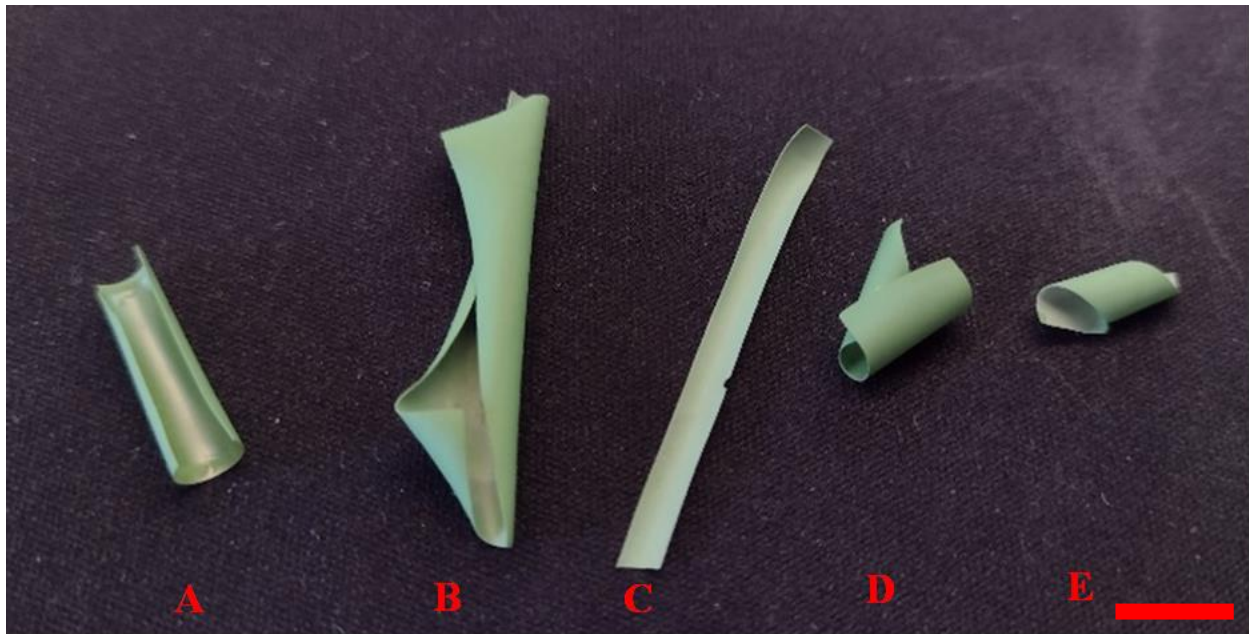
Figure 4.16: SOFC MCCs showing unexpected behaviors. 90^\circ misoriented deformation direction (A, C). Varying local deformation (B, C, D). \sim 45^\circ misoriented deformation direction (E). Scale bar is 5 mm. Adapted from [171].
