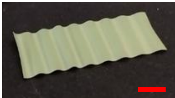
Figure 4.2: Image of wave cell produced using bilayer shrinkage driven self-shaping. Scale bar is 5 mm.
