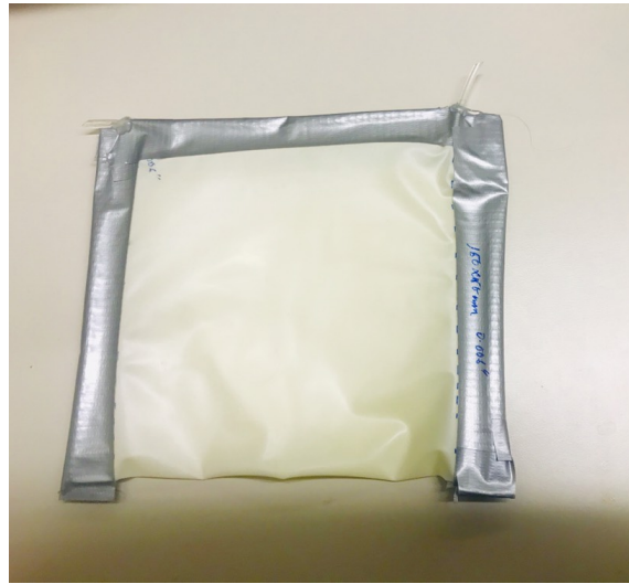
Figure 14: Natural rubber square membrane of 0.006" thickness.
