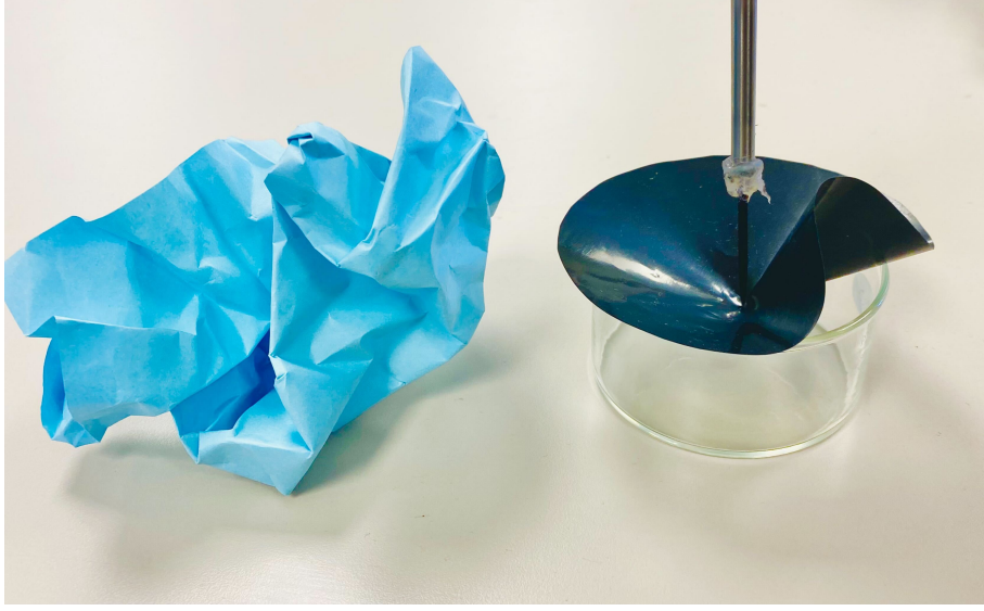
Figure 4: Developable cone: An isolated sharp point on a crushed paper can be thought of as a d-cone, constructed by indenting the center of a circular sheet resting on a hoop.
