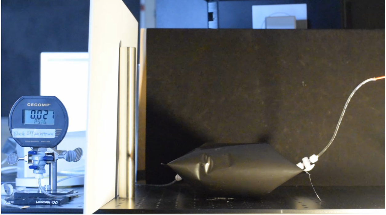
Figure 10: Inflating membrane experiment is recorded using DSLR camera with the corresponding pressure measured using pressure gauge
