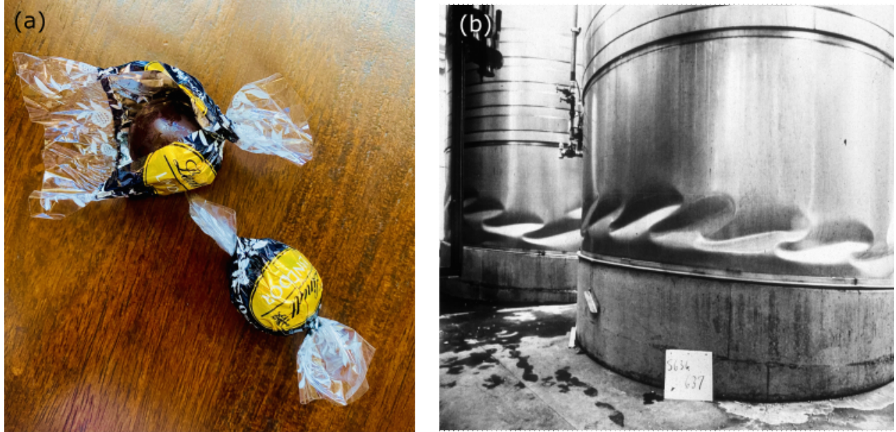
Figure 3: Crumpling in various systems (a) Crumples form on Candy wrappers by twisting a flat sheet around the candy. (b) Crumpling in stainless steel wine tank caused by earthquake. [12]
