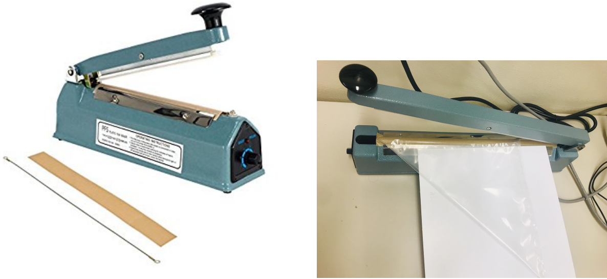
Figure 13: (a)Heat impulse sealer. (b)Heat impulse sealer with a heat sealed LDPE membrane.
