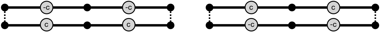
Figure 1.5: The flattened four bar linkage with stress values labeled on each bar. Dotted lines indicate vertices that are connected. Bars have been drawn on two levels for visualization purposes.
