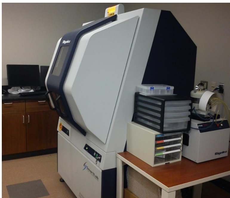
Figure 3. 1 Rigaku SmartLab diffractometer equipment used for XRD analysis
