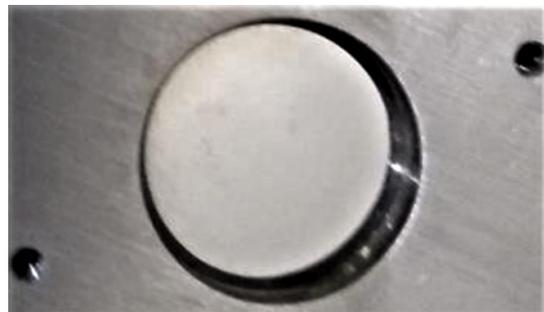
**Figure 4.20:** Photo of 10 $\mu$ m foil taken after the PREX-II experiment had concluded. Foil appears to be in excellent shape.
