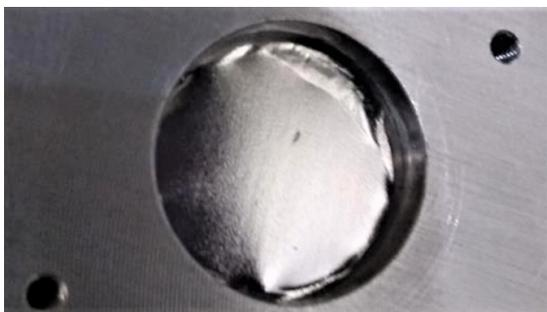
**Figure 4.19:** Photo of 4 $\mu$ m foil taken after the PREX-II experiment had concluded. Foil wrinkling is clearly visible.
