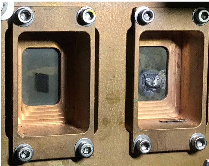
**Figure 2.6:** Post-experiment photo of PREX-II  $^{208}\text{Pb}$  targets. Left-target shows signs of minor thermal wear in the shape of the raster. Right-target shows a target which reached thermal failure.
