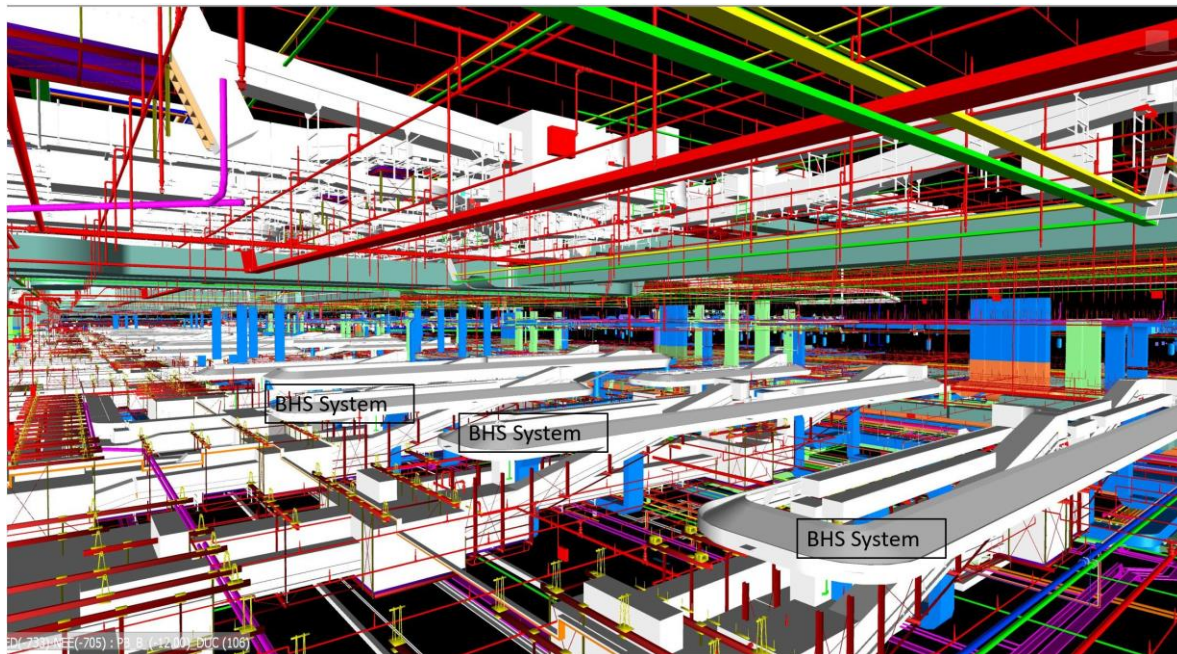
Figure 12. Viewpoint of the Cross-coordination of BHS Systems and MEP Elements within the Terminal Building Zone
