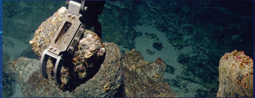
Hercules (above) passes through a swarm of mackerel while exploring Gorringer Bank. With its robotic arm (inset), Hercules reaches out and samples a rock with its jaws, which are about 1 foot long.
