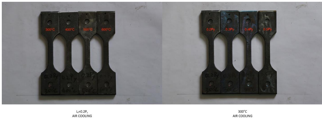
Figure 4-23 Post-fire Surface Conditions of Specimens Subjected to Different Axial Tensile Loads
