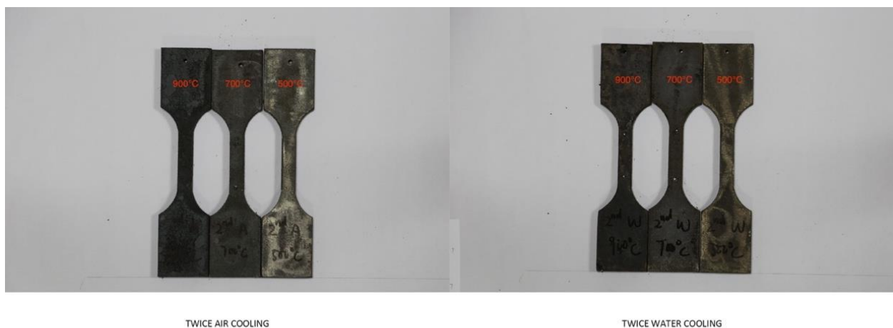
Figure 4-19 Post-fire Surface Conditions of Specimens after Repeated Heating/Cooling
