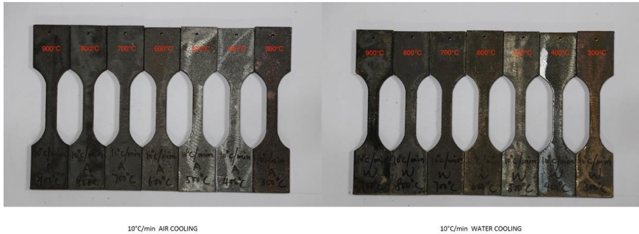
Figure 4-8 Post-fire Surface Conditions of the Specimens Using Different Cooling Methods
