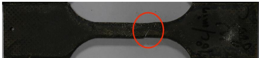
Figure 4-30 Non-ductile Fracture Failure without Necking
