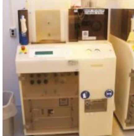
9. Etch the silicon wafer using deep reactive ion etcher (DRIE)
