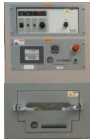
11. Deposit fluoroctyltrichlorosilane (FOTS) on the silicon wafer to make the surface hydrophobic
