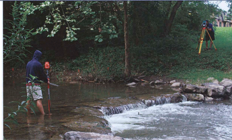
Graduate students Tim Daniluk and Ryan Gordon survey the stream around a restoration structure in Ninemile Creek, Marcellus Park, Onondaga County.
