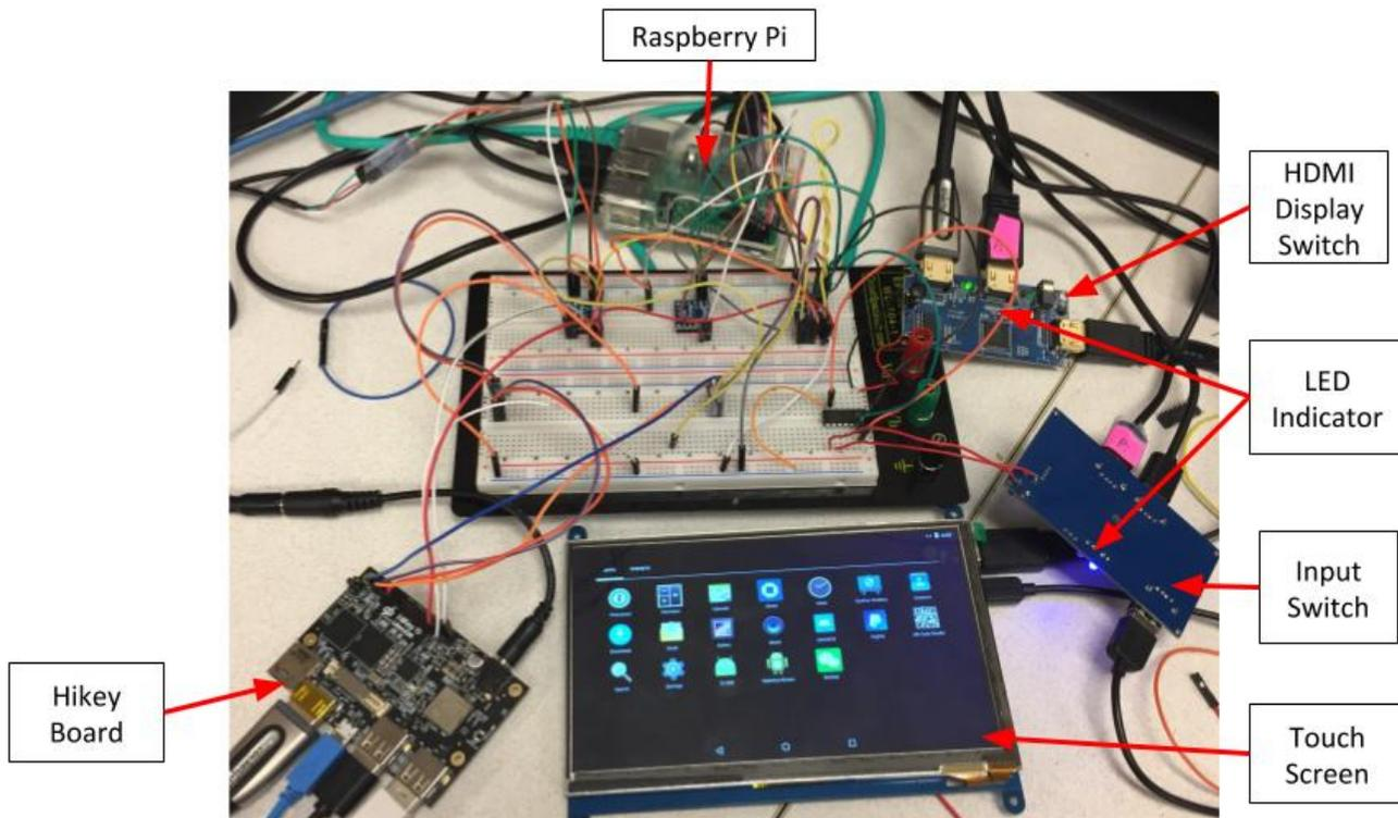
Fig. 3.13.: Hardware Test Setup for Truz-UI
