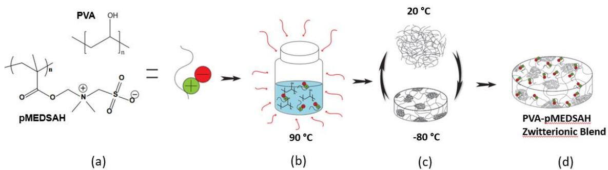
*Fig. 1: Schematic of hydrogel fabrication procedure: (a) Structure of PVA and pMEDSAH (b) Representation of the heating of the PVA-pMEDSAH solution (c) Hydrogel crosslinking process (d) Final hydrogel.*
