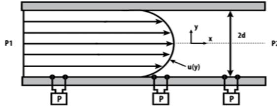
Fig 4: Illustration of the viscosity measurement method.
