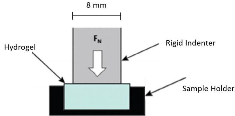
Fig. 3: Illustration of confined compression test set up.
