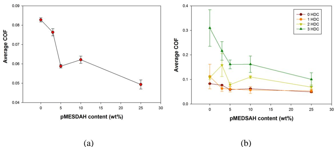
*Fig 7: Friction data for hydrogels with increasing pMEDSAH content (a) Fully hydrated samples with no hydration/dehydration cycles (b) Samples with 0 to 3 hydration/dehydration cycles*
