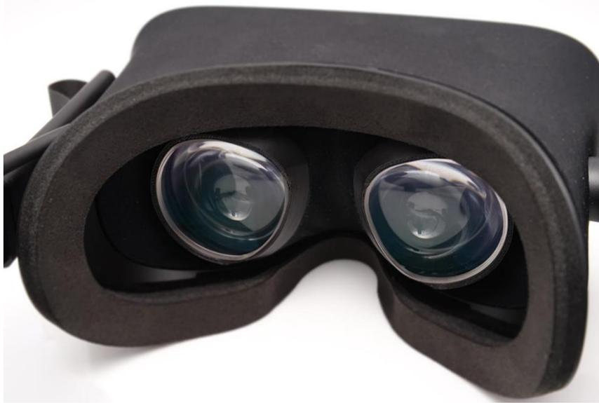
Figure 2. Stereo Lenses for Binocular (stereoscopic) VR Systems (Oculus Rift)
