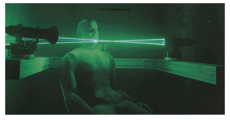
Once particles are introduced into the Indoor Flow Laboratory, researchers use an optical-based technique known as laser Doppler anemometry to collect information on particle velocity, concentration, and flux.
