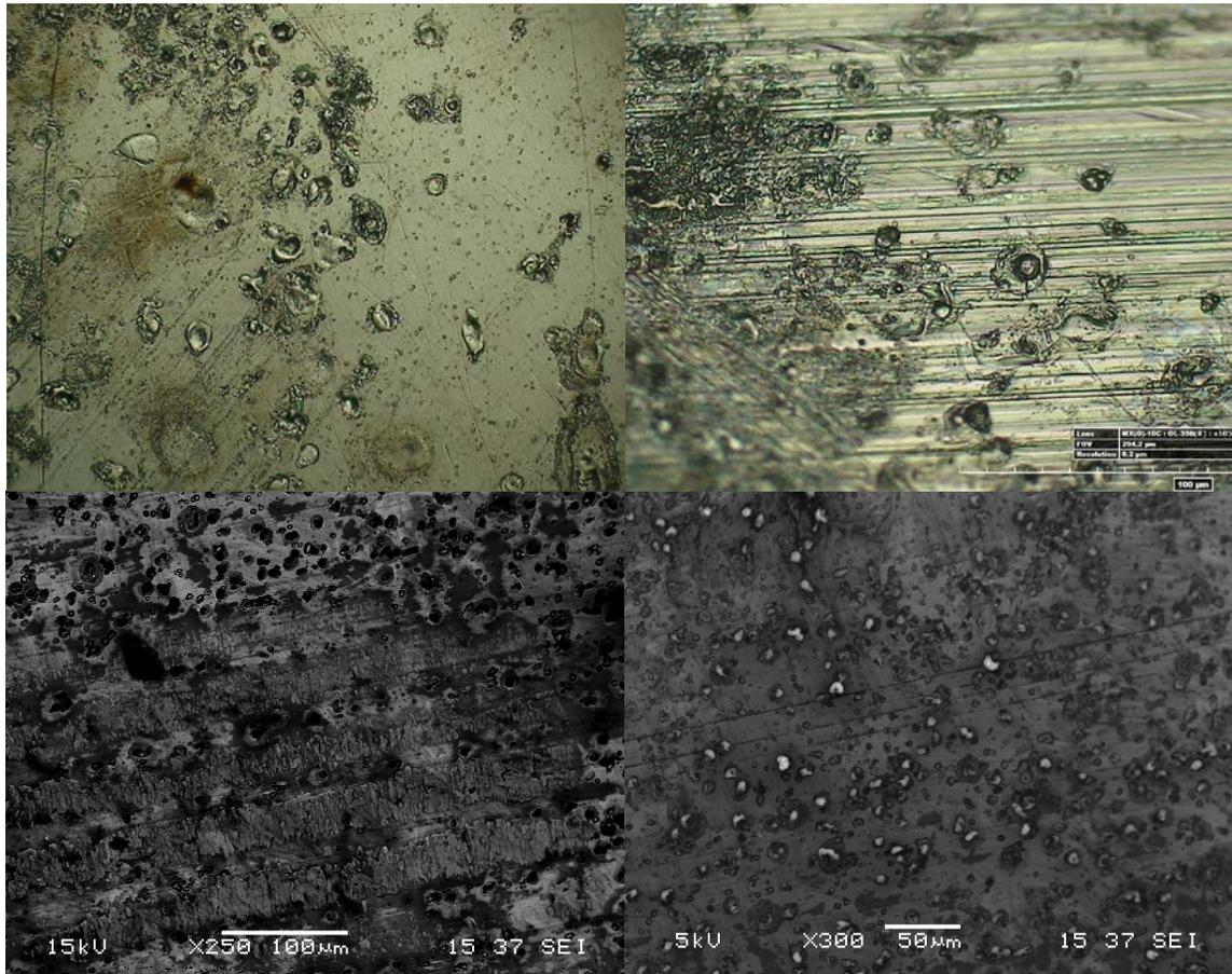
**Figure 1:** Optical microscope image of ICI corrosion surface of CoCrMo liner (A, B). SEM image of ICI corrosion at 15kV(C) and 5kV(D). Note the cell remnants present under 5kV observation (bright regions in D).
