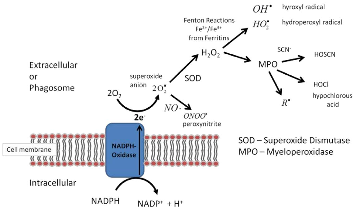
**Figure 2.** Schematic of the oxidative burst reaction. Note, cells make super oxide anions that react into other species ( $H_2O_2$ ,  $HClO$ , etc.), which are reactive with CoCrMo alloy surfaces [9].
