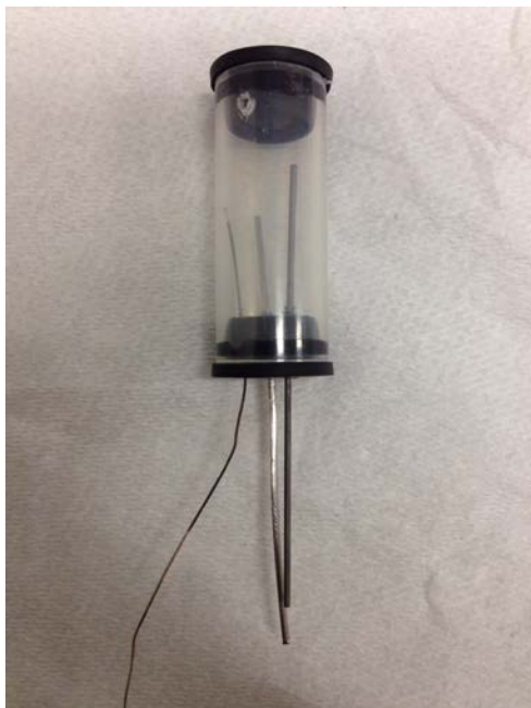
Figure 4: Assembled cell with hole near top for gas exchange.
