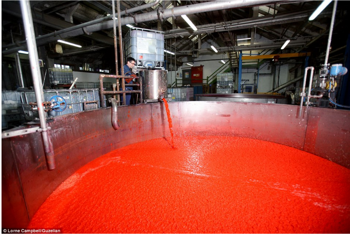
Figure 11: The vat of red dye and paper mulch at James Cropper's factory (Duell 2014; photo courtesy of Lorne Campbell).
