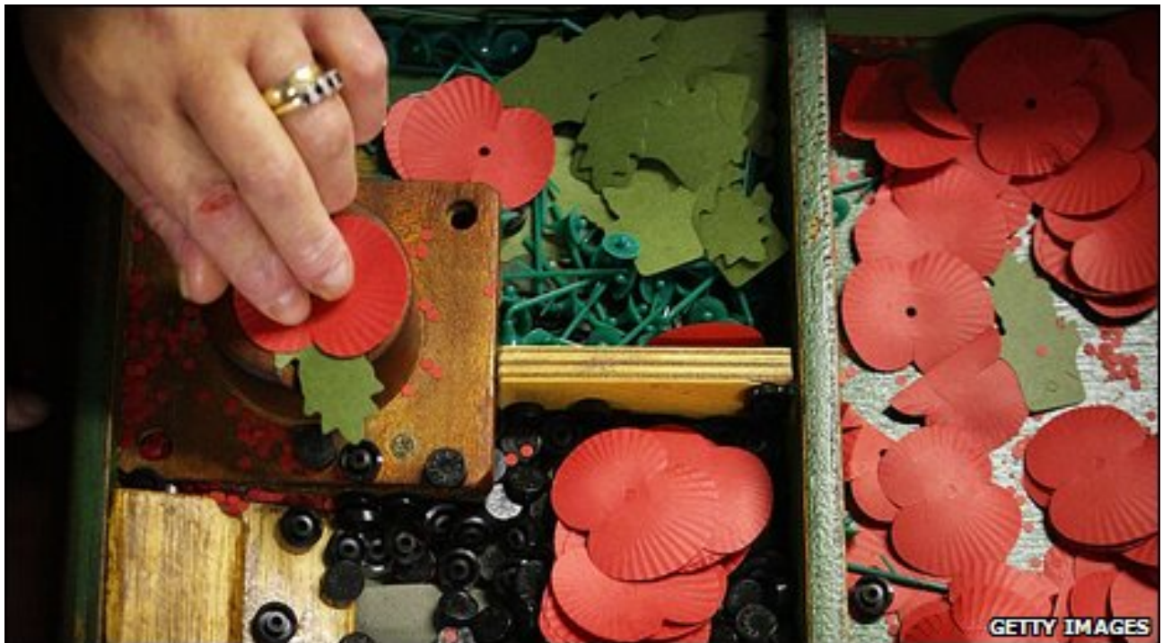
Figure 10: An example of a wooden block that would have enabled soldiers with one arm to assemble the poppy (Mower 2009; photo courtesy of Getty Images).
