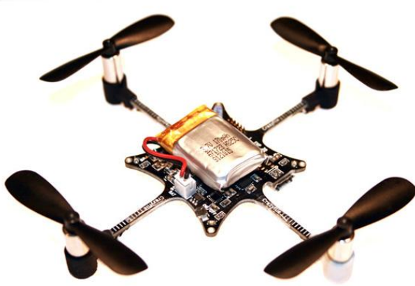
Figure 2. Photograph of the Crazyflie Nano Quadcopter, showing the frame, battery, and set of four blades. [3]
