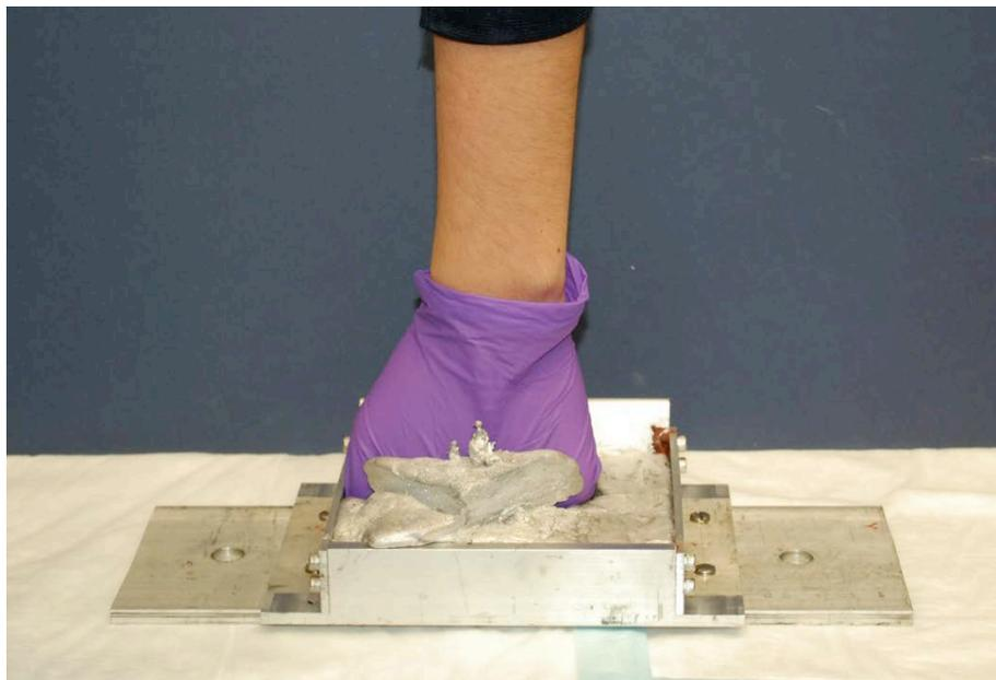
Figure 6b. Wrist Position in Neutral Potting Fixture with Metal Alloy for Molding of the Hand
