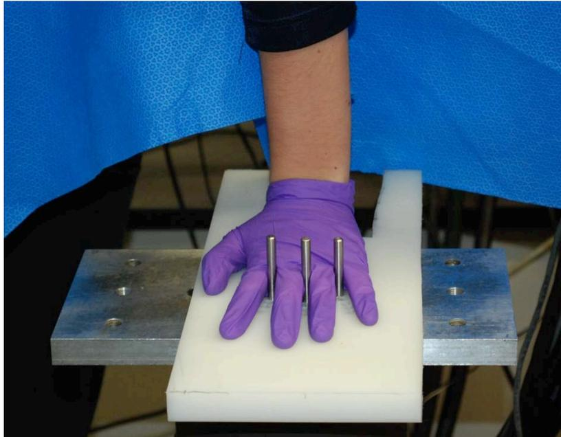
Figure 6a. Wrist Position in MTS during Testing in Extension using Polymer Board with Adjustable Dowel Placement
