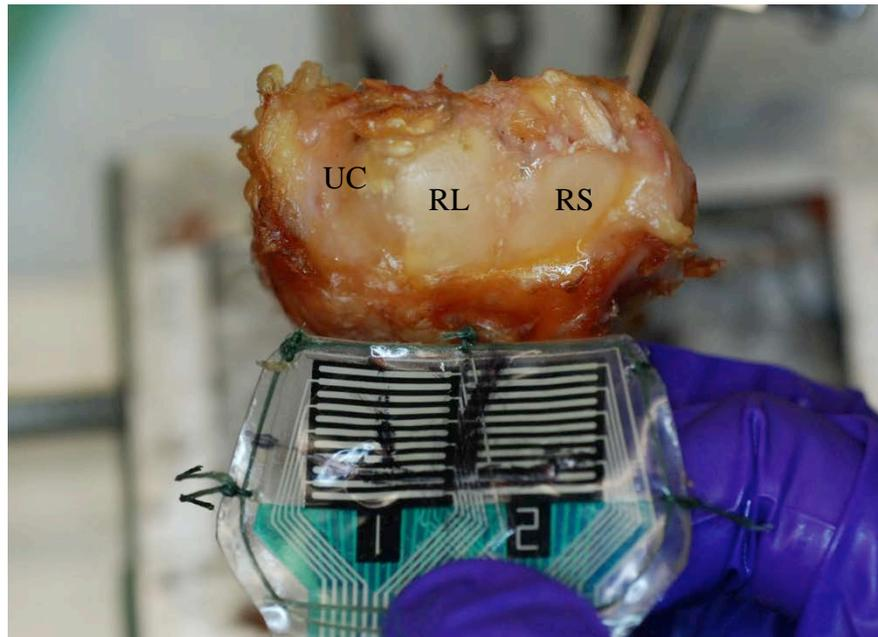
Figure 8. Pressure Sensor after Removal from the Wrist. Lines Drawn on the Sensor Indicate the Borders of the Radiolunate Fossa (RL), Radioscaphoid Fossa (RS), and Ulnar Carpal Fossa (UC) when it was Anchored to the Distal Radius and Ulna
