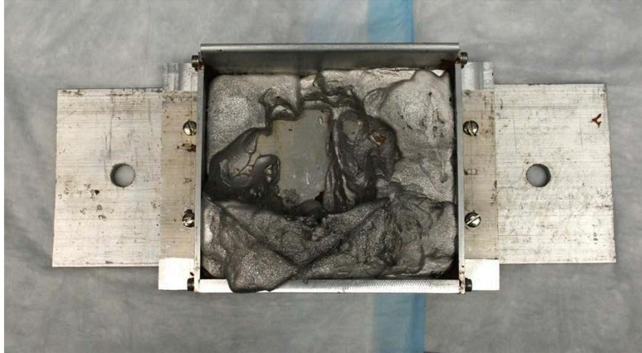
Figure 6c. View from Above of Metal Alloy Mold for the Hand
