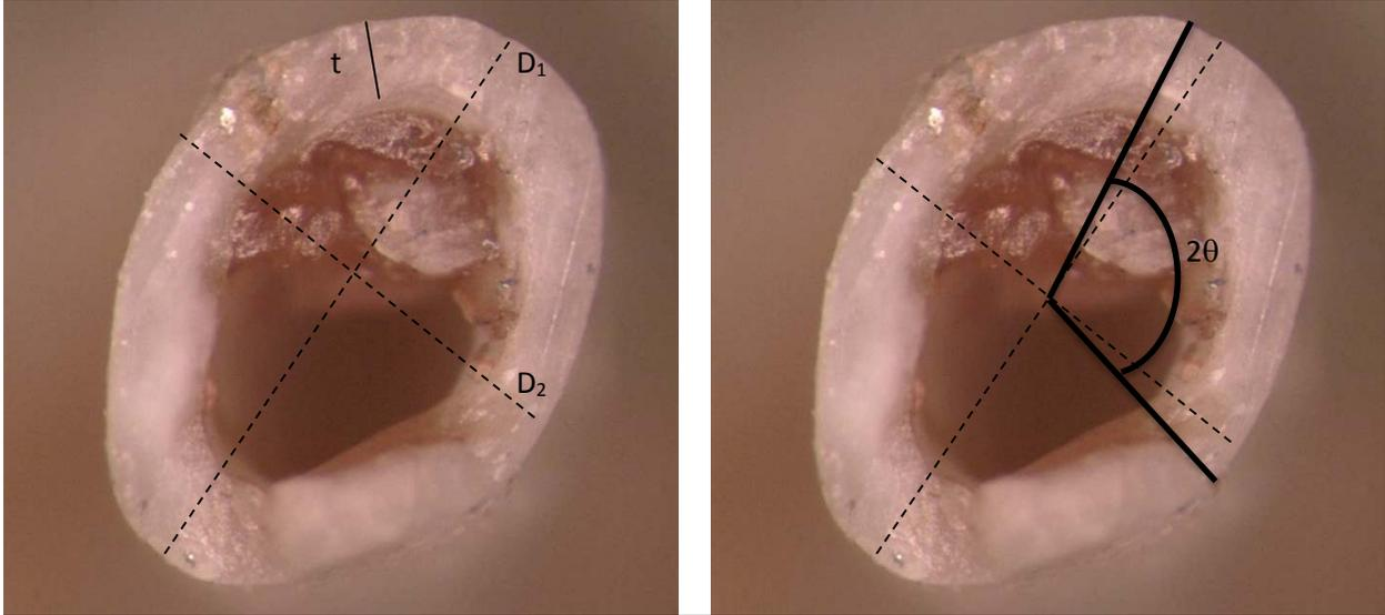
**Figure 3.** Cross-section of bone. Left. Measurements taken from the cross sectional images. D1 is the larger elliptical diameter, D2 is the smaller elliptical diameter. These values were averaged to obtain  $R_o$ .  $t$  is a sample thickness measurement. 4-6 thickness measurements were averaged to obtain a thickness value. Right. The initial crack angle  $2\theta$ . The half crack angle  $\theta$  was calculated using methods described.
