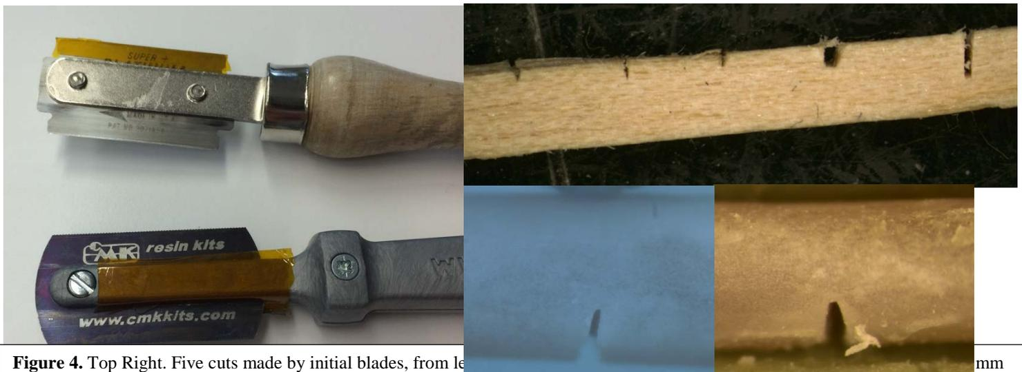
**Figure 4.** Top Right. Five cuts made by initial blades, from left to right: two serrated, one hybrid, and two razor. Bottom Right. Cut made by “hybrid” polisher-filed blade. Bottom Middle. Final notch design made from using the filed serrated blade and the thinner razor blade. Left. Two blades used for notching. The bottom blade is serrated to aid ease of notching and was filed on a polisher to reduce width. The top blade is thinner and was used to add a sharp tip to the notch. mm
