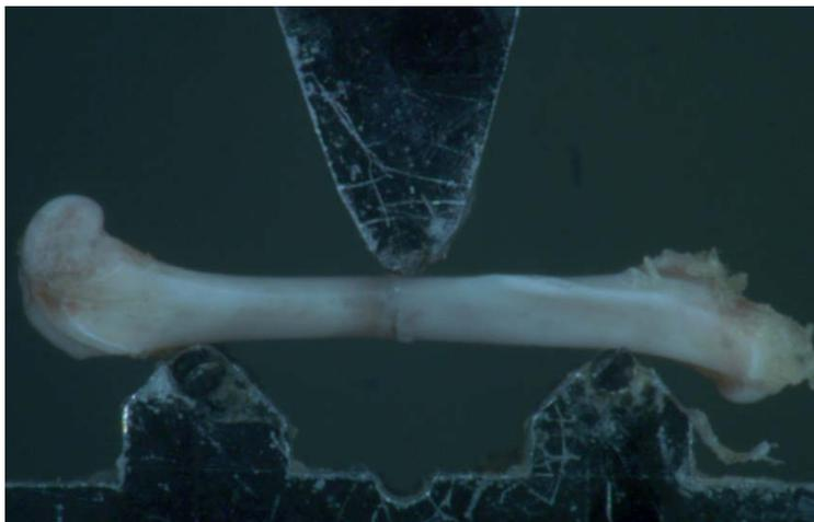
**Figure 2.** Testing set up. Bottom right: the entire testing set up from L to R: QTest machine with 3-pt bend set up, camera stabilized by a foam piece to prevent shaking of the images during testing, function generator set to a 1 Hz square wave. Bottom Left: 3-pt bend set up with light system and camera lens. Top Left: a notched, tested bone in the 3-pt bend set up. Bone is noted on anterior side and places anterior side down in the testing set up. Bottom supports have an 8mm span.
