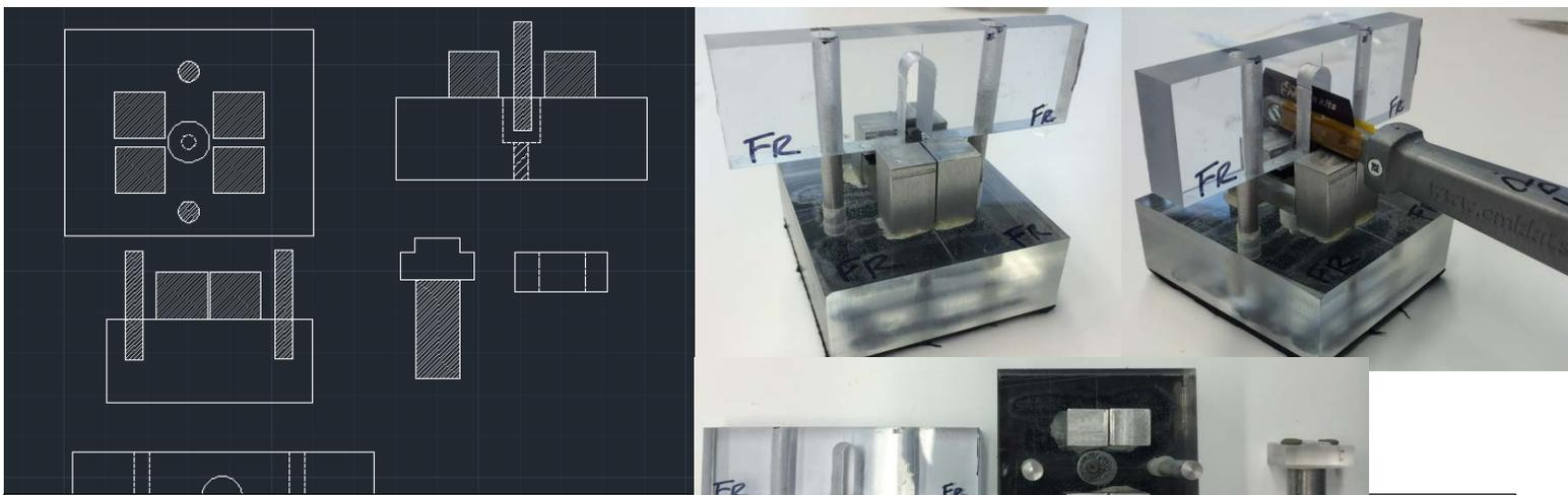
Figure 1. Left. AutoCAD representation. Top and two side views and the aluminum components indicated by narrow gray hatching. Right. Three views of the notching device. Clockwise from top left: notching device assembled for notching, no blade, notching device assembled for notching with blade, notching device in parts. Clay used for holding bone in position can be seen on the pedestal at the right of the bottom picture.
