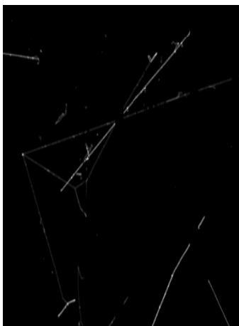
(a) Pion reconstructed track range is less than 75 cm and longer than muon track due to dead wires
