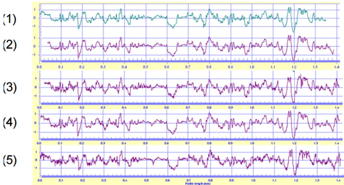
Measurement comparison of four techniques tracing the same SRM bullet:
