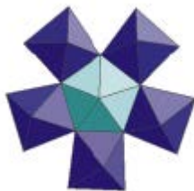
Fig. 5: Polyhedral representation of the \{\text{Mo}\}\text{Mo}_5 unit present in Mo-132. In the center (light blue) is a \{\text{MoO}_7\} pentagonal bipyramid, surrounded by five \{\text{MoO}_6\} octahedra (dark blue), all of which are linked the central polyhedron through edge sharing. 37
