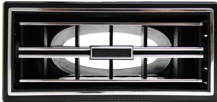
Figure 6-3 Diffuser with louvers installed
