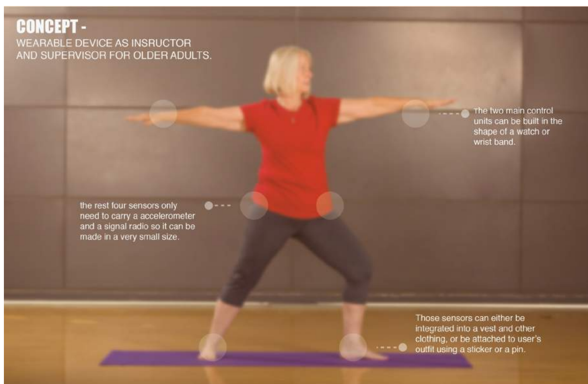
Fig. 4. Initial concept design of the wearable device as a personal electronic exercise instructor.
