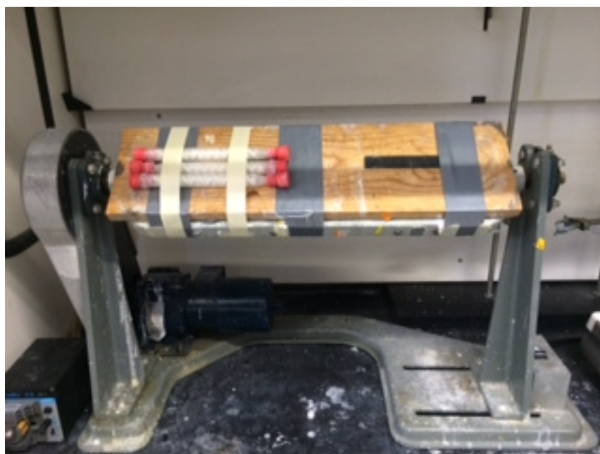
Figure 2: Coated mixing nozzles on the rotating drum during the first 20 hours of the coating process (both ends are sealed with a rubber stopper).
