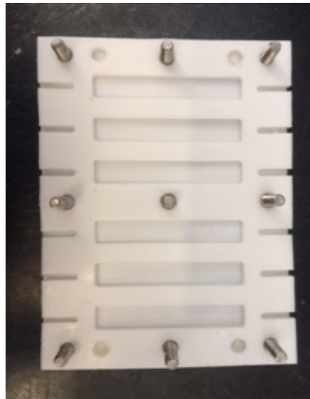
Figure 7: Flexural test sample mold with six channels.
