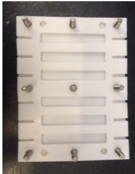
Figure 7: Flexural test sample mold with six channels.
