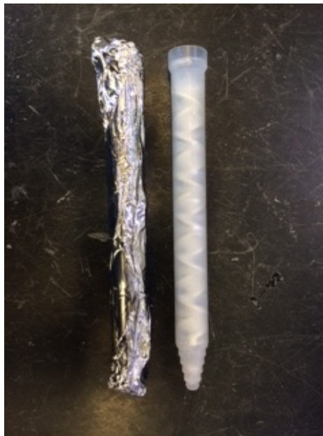
Figure 3: A covered and uncovered coated mixing nozzle before being stored.
