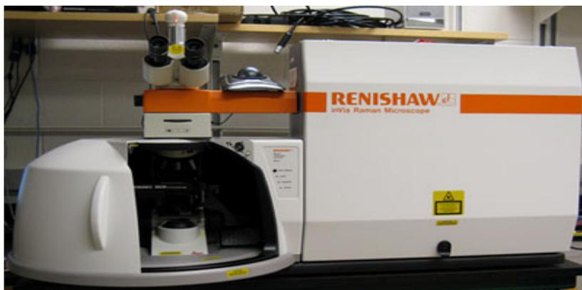
Figure 10: Renishaw inVia Raman microscope
