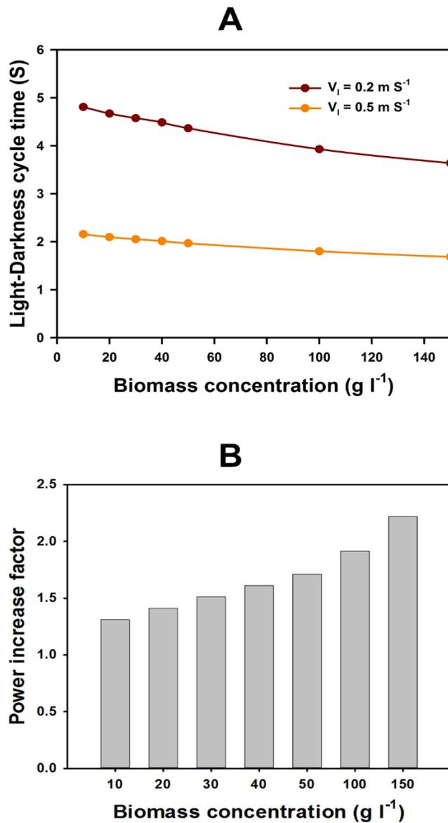
**Figure 5.2: Application of the rheological properties of microalgal broths for flow manipulation.** Light-darkness cycle time  $t_c$  determined at different biomass concentrations using the flow properties (A) and the power consumption with an axial velocity of  $0.5 \text{ m} \cdot \text{s}^{-1}$  at different microalgal concentrations (B).
