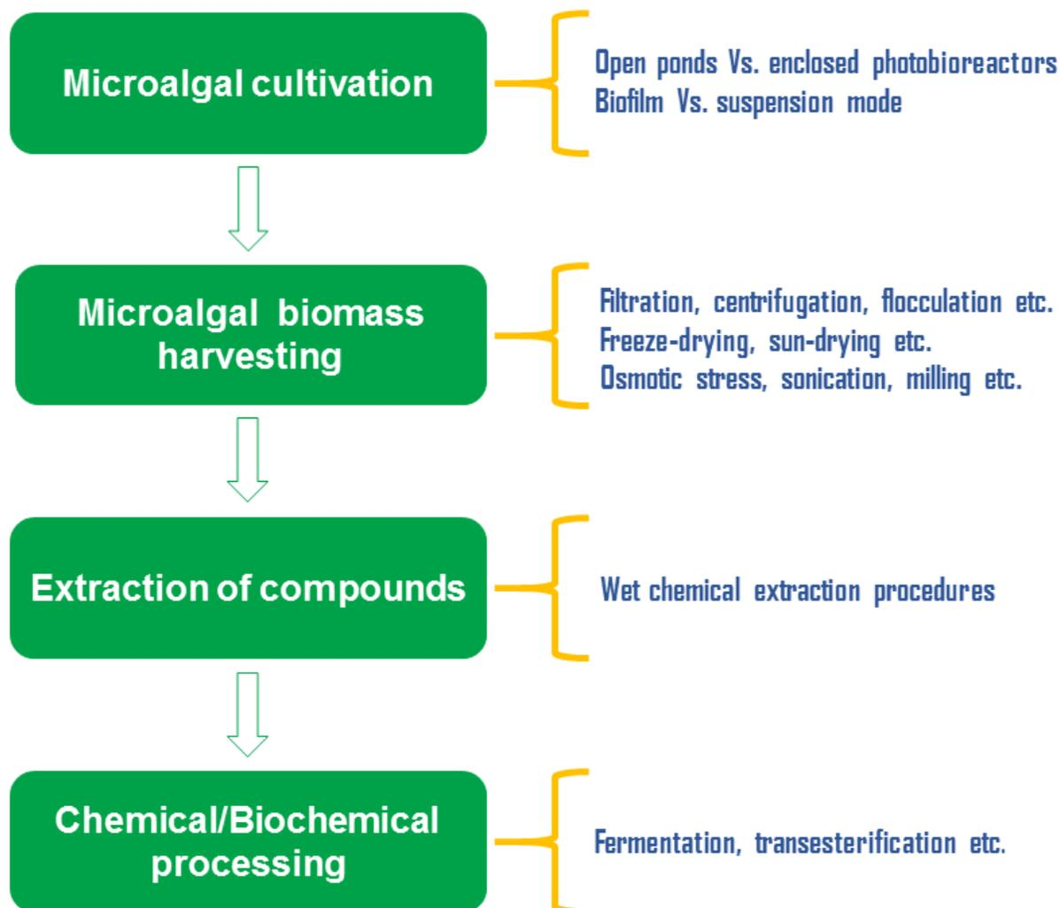
**Figure 1.4: Illustration of microalgal biorefining processes.** Microalgae are first cultured in open or enclosed systems. Then, the microalgal biomass is harvested. This is often followed by the extraction of the valuable compounds and further chemical processing to obtain the target specialty chemicals.
