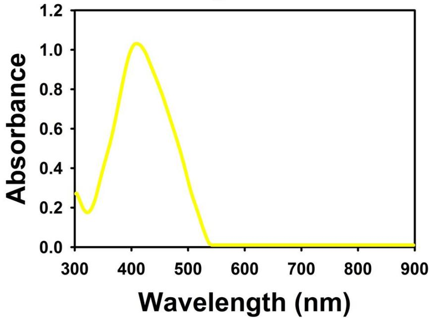
**Figure 2.1: Plasmonic film consisting of silver nanospheres.** Photograph of a plasmonic film after being peeled off from petri-dish (A) and absorbance spectrum of the plasmonic film consisting of spherical silver nanoparticles (B).
