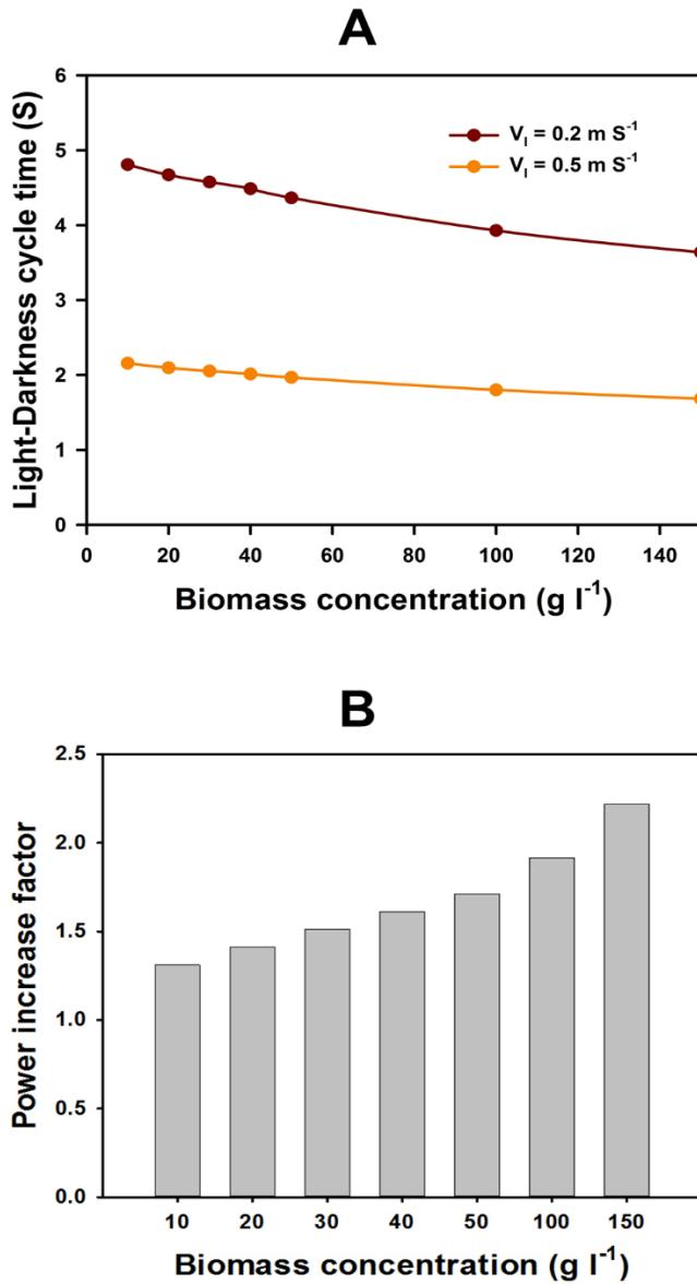
**Figure 5.2: Application of the rheological properties of microalgal broths for flow manipulation.** Light-darkness cycle time  $t_c$  determined at different biomass concentrations using the flow properties (A) and the power consumption with an axial velocity of  $0.5 \text{ m. s}^{-1}$  at different microalgal concentrations (B).
