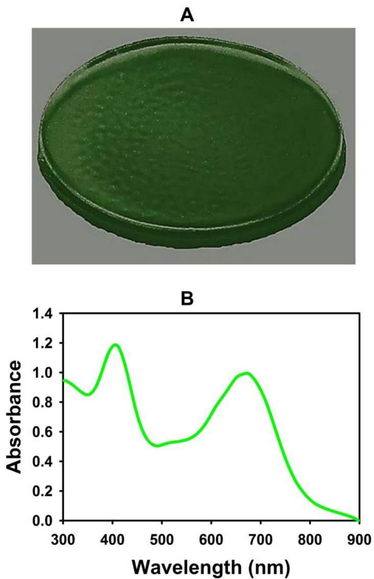
**Figure 2.3: Plasmonic film consisting of silver nanospheres and gold nanorods.** Photograph of a plasmonic film consisting of gold nanorods and silver nanospheres after being peeled off from petri-dish (A) and absorbance spectrum of the plasmonic film consisting of gold nanorods and silver nanospheres (B).
