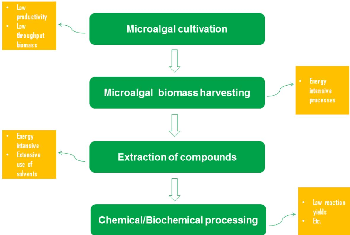
**Figure 1.3: Illustration of current challenges in microalgal biomass production and biomass processing.** The most critical issues include the low productivity and the high energy consumption in each step.
