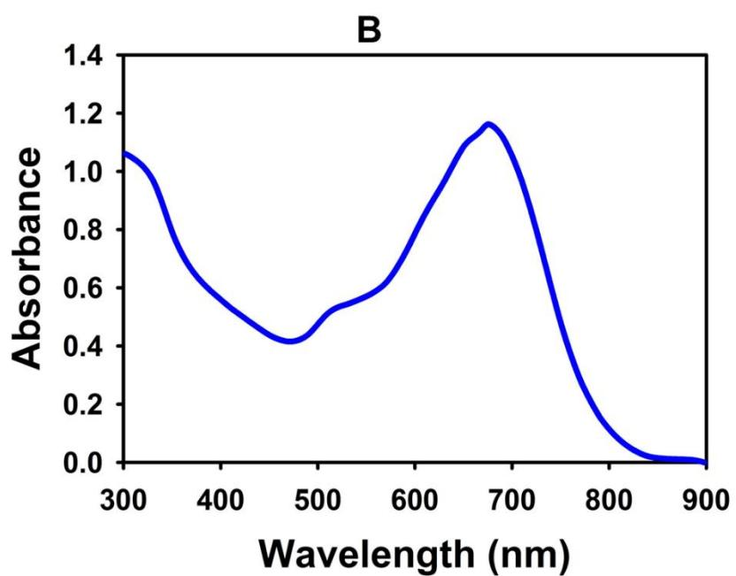
**Figure 2.2: Plasmonic film consisting of gold nanorods.** Photograph of a plasmonic film consisting of gold nanorods after being peeled off from petri-dish (A) and absorbance spectrum of the plasmonic film (B).
