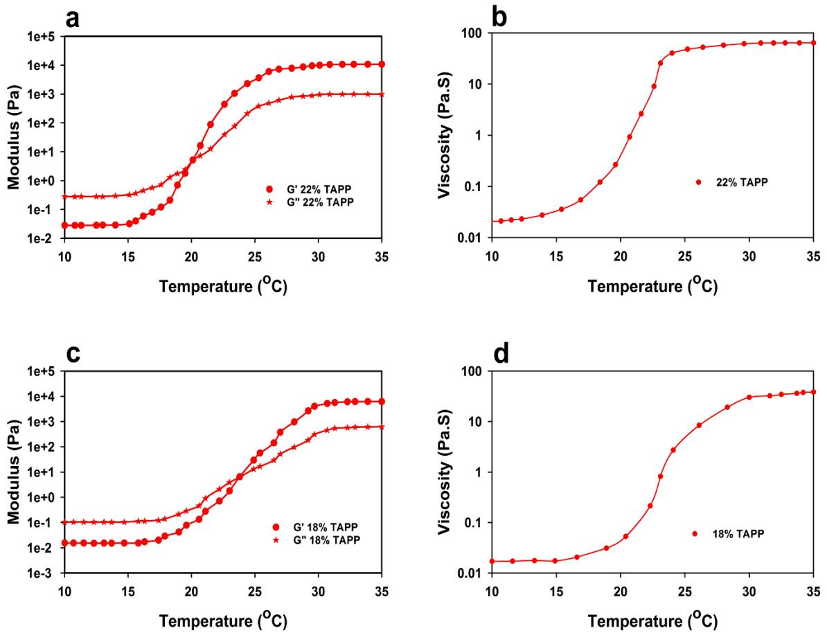
**Figure 3.2: Thermorheological properties of the TAPP medium.** (a) Storage modulus (circle) and loss modulus (star) of the 22% pluronic in TAPP sample as a function of temperature, (b) viscosity profile of the 22% pluronic in TAPP sample as a function of temperature, (c) storage modulus (circle) and loss modulus (star) of the 18% pluronic in TAPP sample as a function of temperature and (d) viscosity profile of the 18% pluronic in TAPP sample as a function of temperature.
