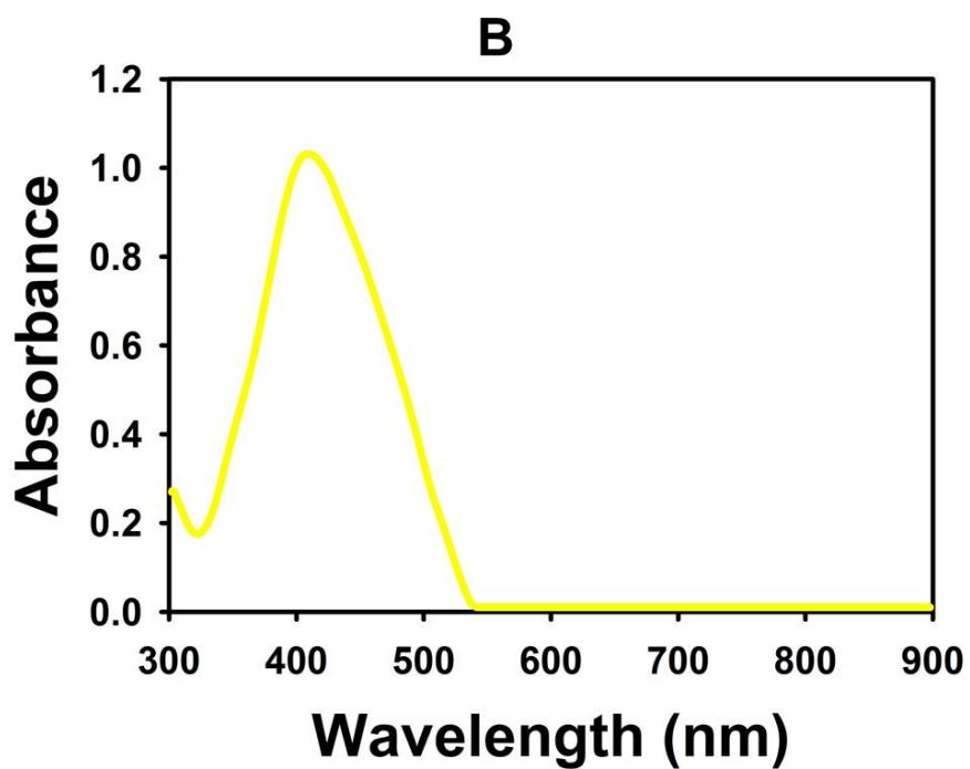
**Figure 2.1: Plasmonic film consisting of silver nanospheres.** Photograph of a plasmonic film after being peeled off from petri-dish (A) and absorbance spectrum of the plasmonic film consisting of spherical silver nanoparticles (B).
