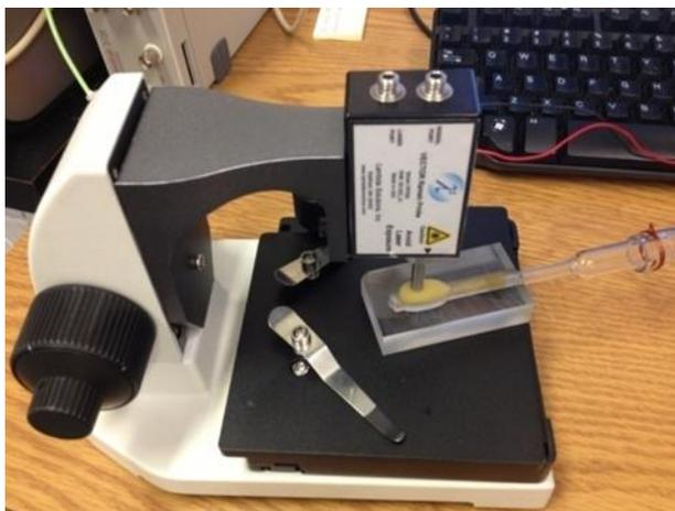
**Figure 4.2.** Lambda Solutions probe mounted on microscope base with probe contacting a latex bulb whose internal pressure can be monitored. The rat paw is placed in between the probe and bulb, palm up.
