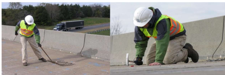
Figure 2-1 Chain drag and hammer testing (SHRP2, 2015)
