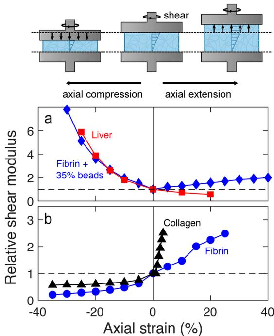
**FIG. 1.** Stiffening and softening in uniaxial strain. The shear modulus, measured within the linear regime (shear strain  $\sim 2\%$ ) is shown as a function of the applied axial strain for (a) liver and a composite of fibrin embedded with polysaccharide beads, and for (b) reconstituted networks of purified fibrin and collagen. Data adapted from Ref. 14.
