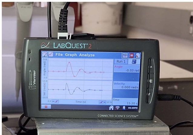
Fig 6. Sample snapshot of a completed data readout on LabQuest. The 2 displayed curves are (top) angular position in radians and (bottom) angular velocity in rad/s, both shown with time on the x-axis. A small, brief twist was made on the top plate at the moment both quantities deviate from zero, and the sample displayed the decaying oscillations shown in response. The red and blue circles guide the eye to equally spaced moments in time but were not used for analysis. The time and magnitude of the peaks in angular position can be found with the LabQuest by using the left arrow and right arrow buttons seen toward the bottom of the screen to move the crosshairs from point to point, or the data can be read in software on a connected computer.
