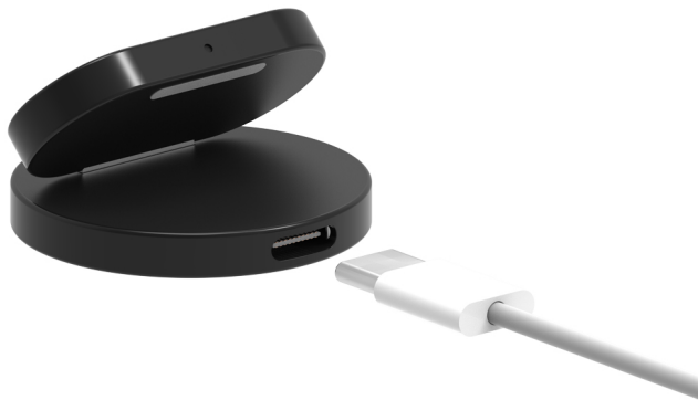
Figure 63. This Rendering Shows that Users Can Charge the Camera Via A USB-C Cable.
