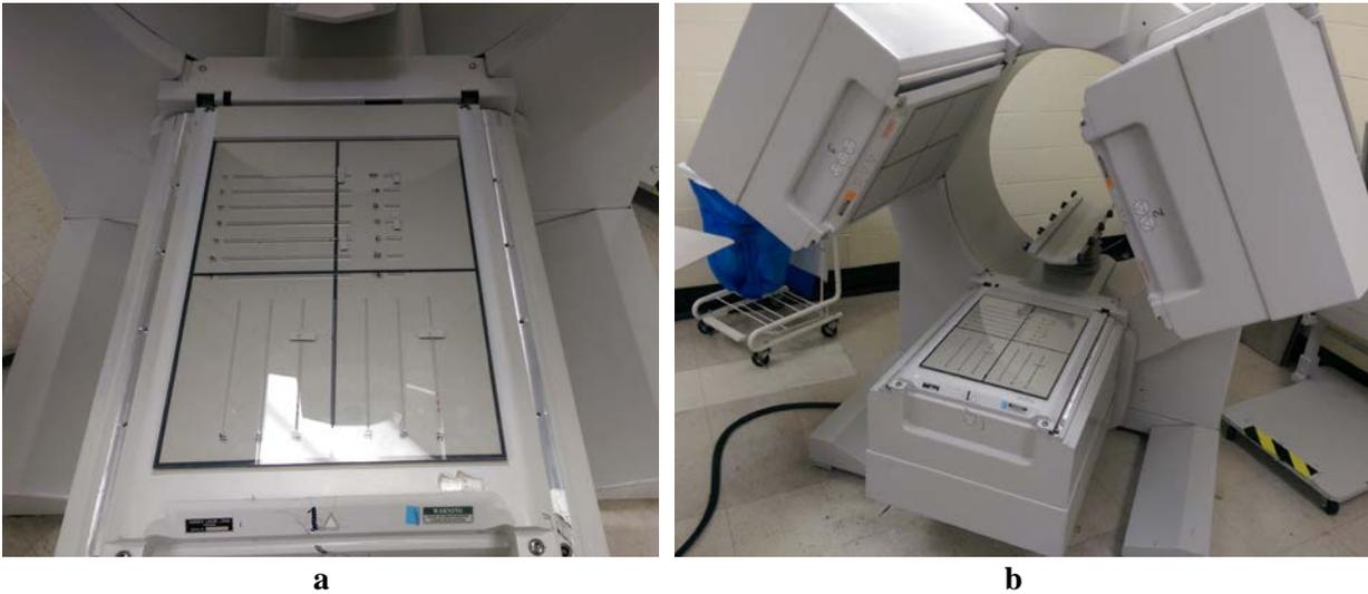
**Fig. 3.2.** Experiment setup for (a) Siemens e.cam dual-head camera with LEHR parallel beam collimators, and (b) Trionix Triad triple-head camera with LEHR fan beam collimators. Courtesy of SUNY Upstate University Hospital.
