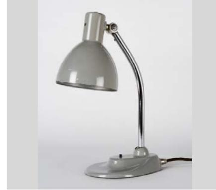
CHROME-PLATED BRASS ARM, NICKEL-PLATED BRASS JOINTS, SHEET STEEL REFLECTOR PAINTED GREY, PAINTED ALUMINUM BRONZE ON THE INSIDE, CAST IRON BASE AND PAINTED GRAY OVER SHEET STEEL BASE PLATE
