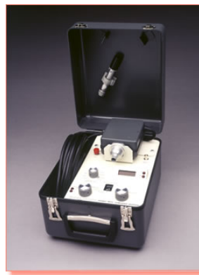
Figure 2: The MDH Industries Model 1015 radiation monitor used in this study with the 10X5-6 ion chamber attachment disconnected, housed in the instrument's cover [7]
