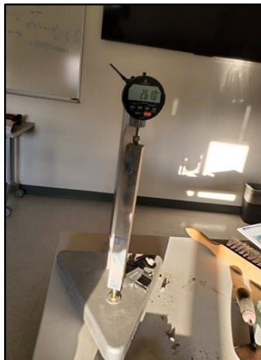
Figure 2.2 Using Length Gauge to Determine the Change of Length with Time
