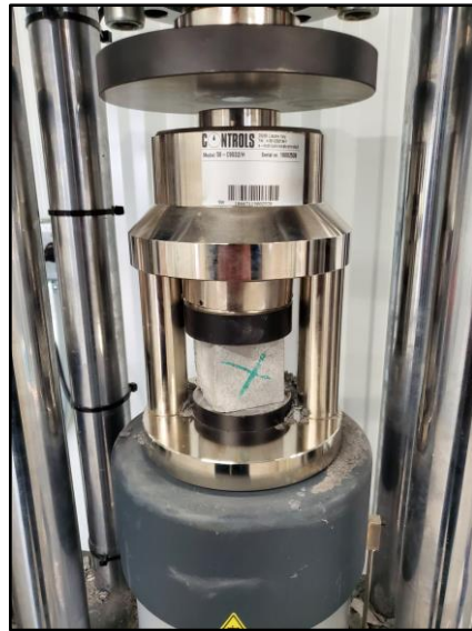
Figure 2.3 Measuring the Cement Mortar Compressive Strength Using an Automated Machine
