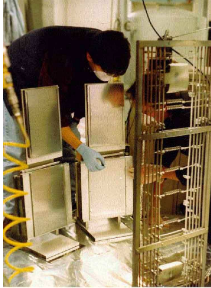
Fig. 10. The coating chamber for sputtering the metallized strips on the \text{CaF}_2 windows. In the foreground are the tungsten filaments which will vaporize the silver onto the crystals. The four crystals in the background lay behind steel masks with 100\ \mu\text{m} slots cut into them to define the high voltage traces.
