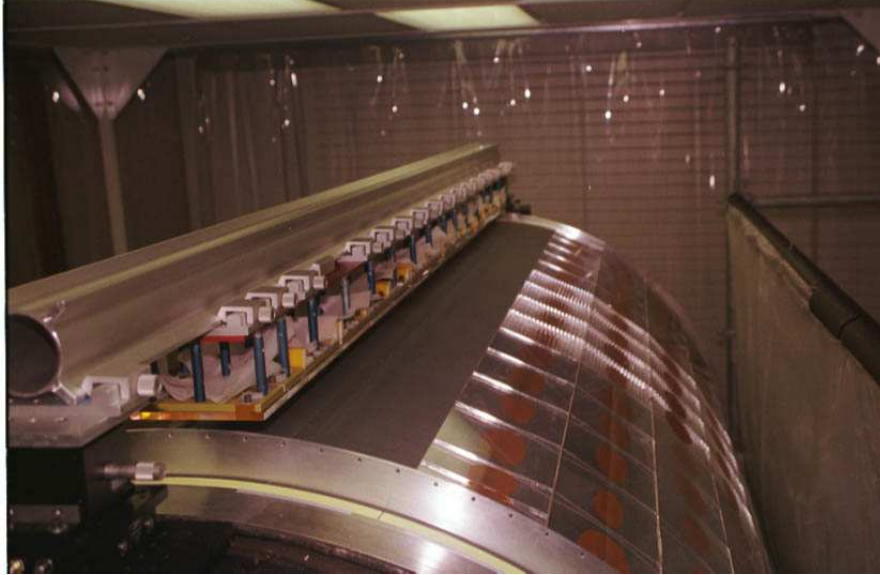
Fig. 22. Photograph of one row of crystal radiators being aligned on the inner carbon fiber cylinder. Previously epoxied rows are shown on the right half of the cylinder. The inner half of the end flange is visible in the forefront.
