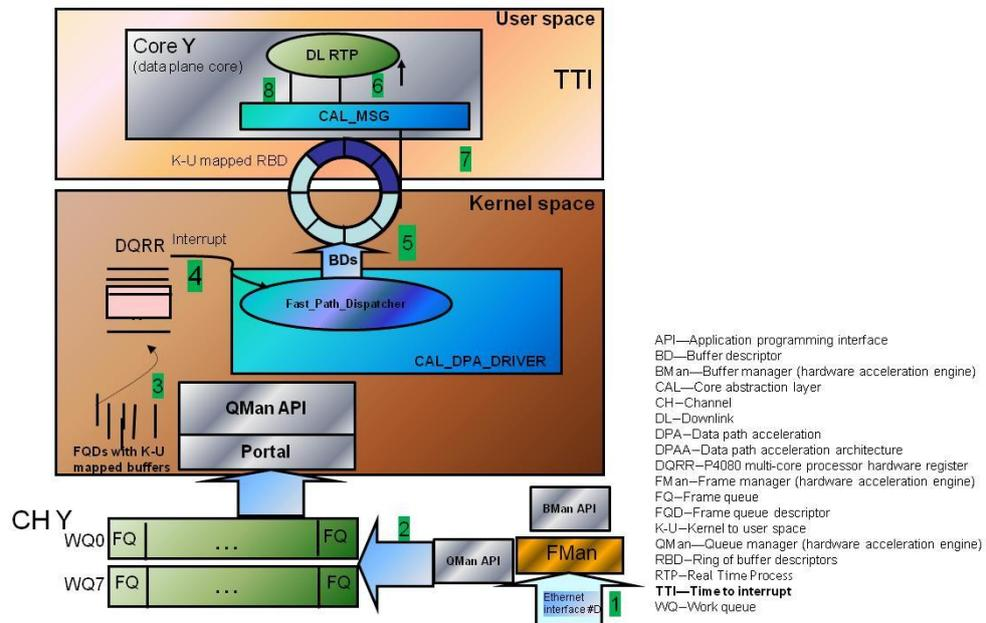
**Figure 19: Ingress Data Plane IP Packet Processing**
