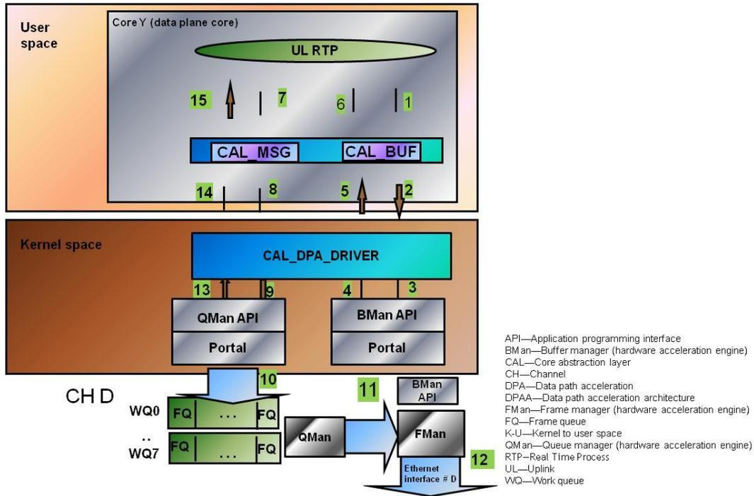
**Figure 20: Egress Data Plane IP Packet Processing**
