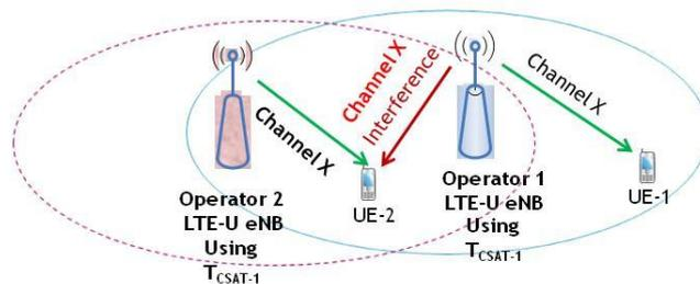
**Figure 3:** Multi-Operator LTE-U Co-channel Interference Scenario
