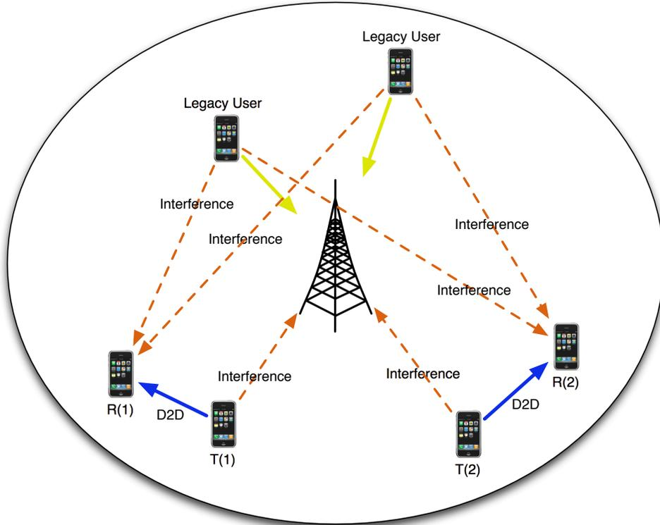
Figure 3-1: A wireless network with D2D links
