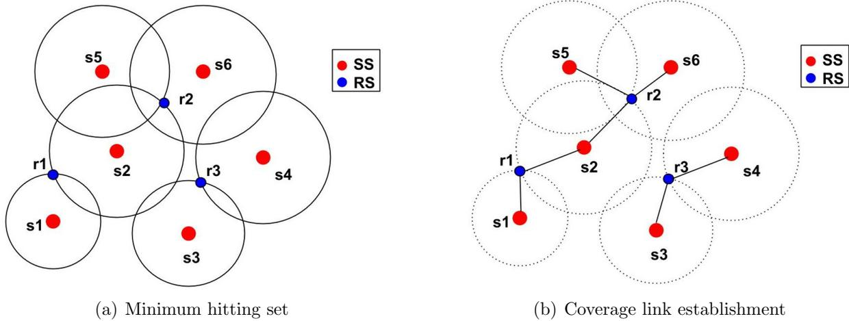
Figure 2-4: Minimum Hitting Set and Coverage Topology
