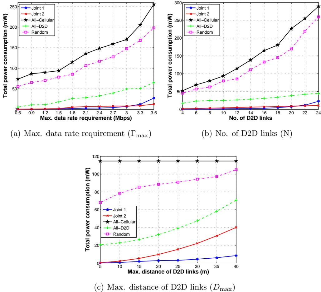
Figure 3-2: Impact of  $\Gamma_{\max}$ ,  $N$  and  $D_{\max}$  on the total power consumption
