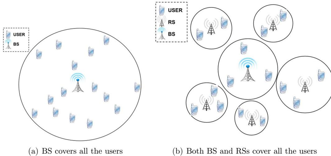
Figure 2-17: Illustration of GREAN design
