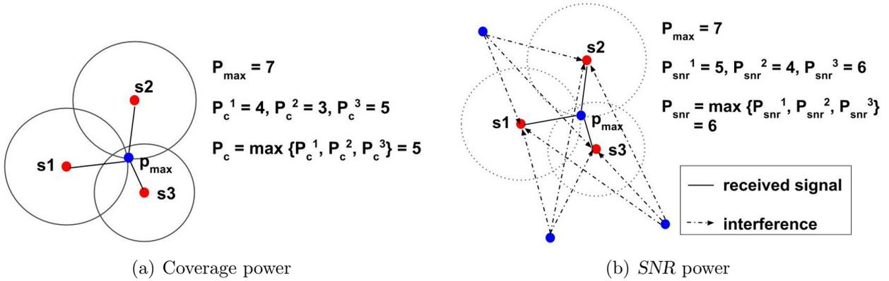
Figure 2-6: Coverage Power and SNR power calculation
