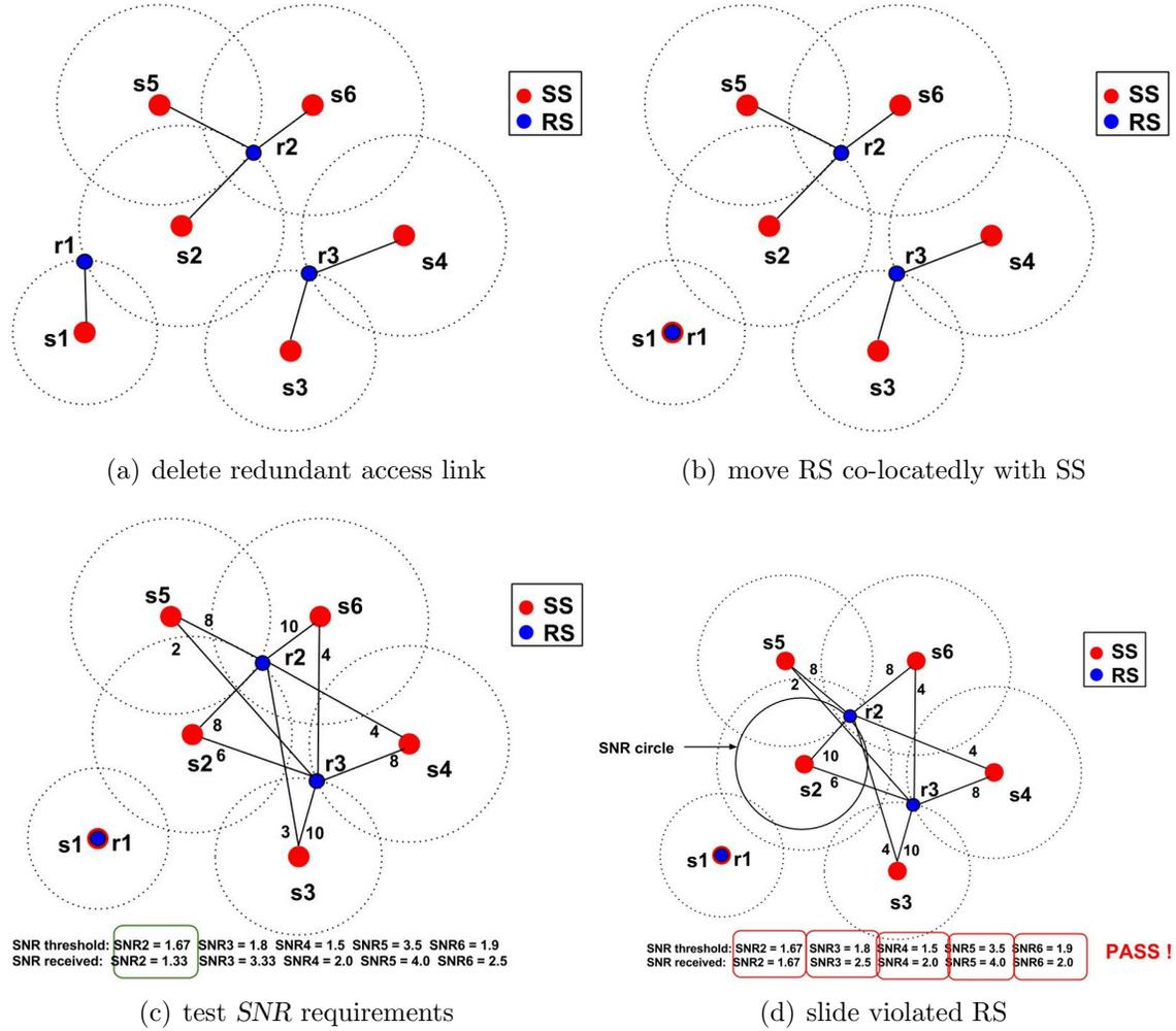
Figure 2-5: Illustration of Coverage Link Escape and RS Sliding Movement
