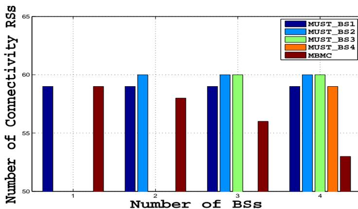
Figure 2-12: Compare the performance between MBMC and MUST with various number of BSs in  $3km \times 3km$  field( $N_{SS} = 300$ )
