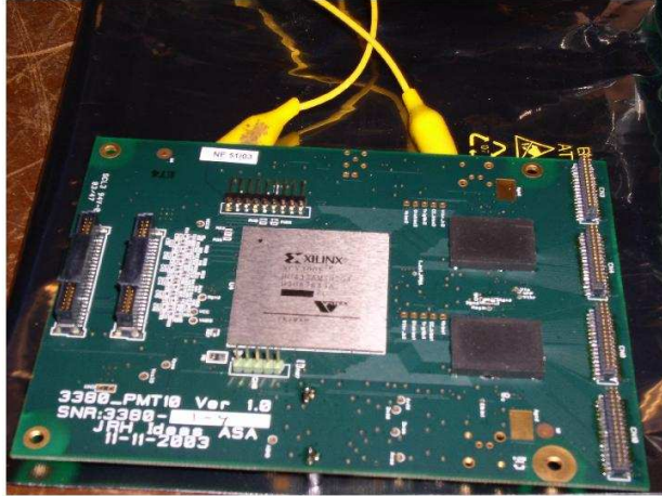
Fig. 16. VA_MAPMT ASICs mounted on the hybrids used in the BTEV gas RICH prototype studied with test beam runs at Fermilab.
