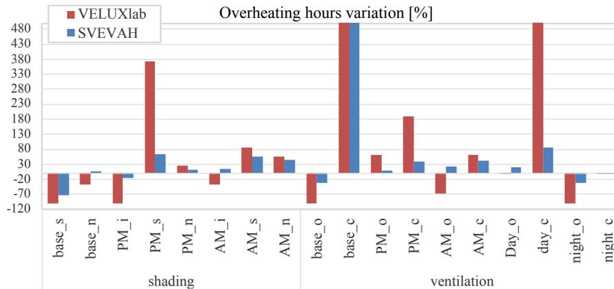
Figure 2. Variation of overheating hours in percentage, calculated according to AH Specifications, 2<sup>nd</sup> edition (2013) ([www.activehouse.info](http://www.activehouse.info)) and compared to baseline scenario.
