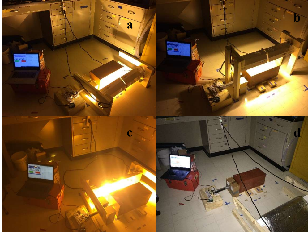
Figure 12: The heating experiment in its four modes: (a) right side heating, (b) top side heating, (c) left side heating, and (d) "nighttime". The apparent light in the 12d is from a camera flash to make the setup visible.
